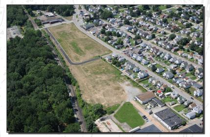
installation of groundwater monitoring wells for long term monitoring. Approximately 100,000 cubic yards of fill material were hauled from an off-site source to construct building PAD areas level with the adjacent roadway and above the FEMA floodplain elevation.
